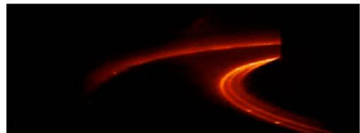
Fig. 3.  $D_\alpha$  filtered tangential X-point TV images show multiple stripes on the inner strike point during the  $n = 3$  I-coil current pulse in shot #123301 at 2171 ms. Only a single stripe is observed both before and after the I-coil pulse.
