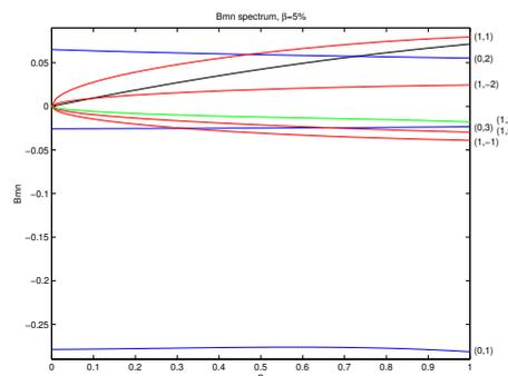
Fig. 4. Radial dependencies of few largest Fourier coefficients  $B_{m,n}$  for optimized configuration.  $B_{0,0}$  is shown by black line and is plotted in the form  $B_{0,0}(s) - B_{0,0}(0)$ , with  $B_{0,0}(0) = 1$ .
