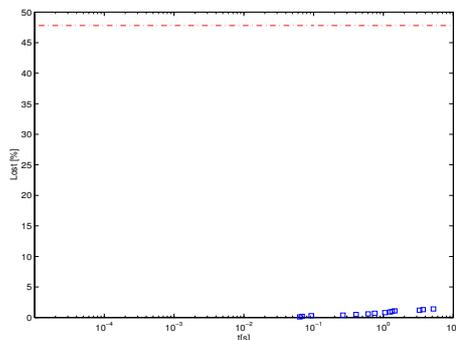
Fig. 3. Collisionless  $\alpha$ -particle confinement in the optimized configuration as a function of the time of flight. One thousand particles are started at  $s_{start} = 0.44$  ( $2/3$  of the plasma radius); the dashed line shows the fraction of the reflected particles.
